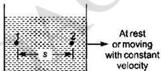
(b) Pressure at two points which are at a depth separation of  $h$  when fluid is at rest or moving with constant velocity is related by the expression
